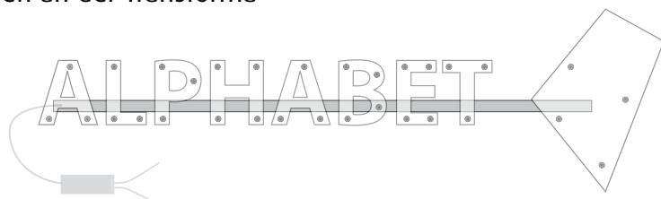
5. Place the front at the right position and screw the front of the sign to the backplate with the small screws. With this type of mounting, no water will enter the sign and it keep dirt outside.
